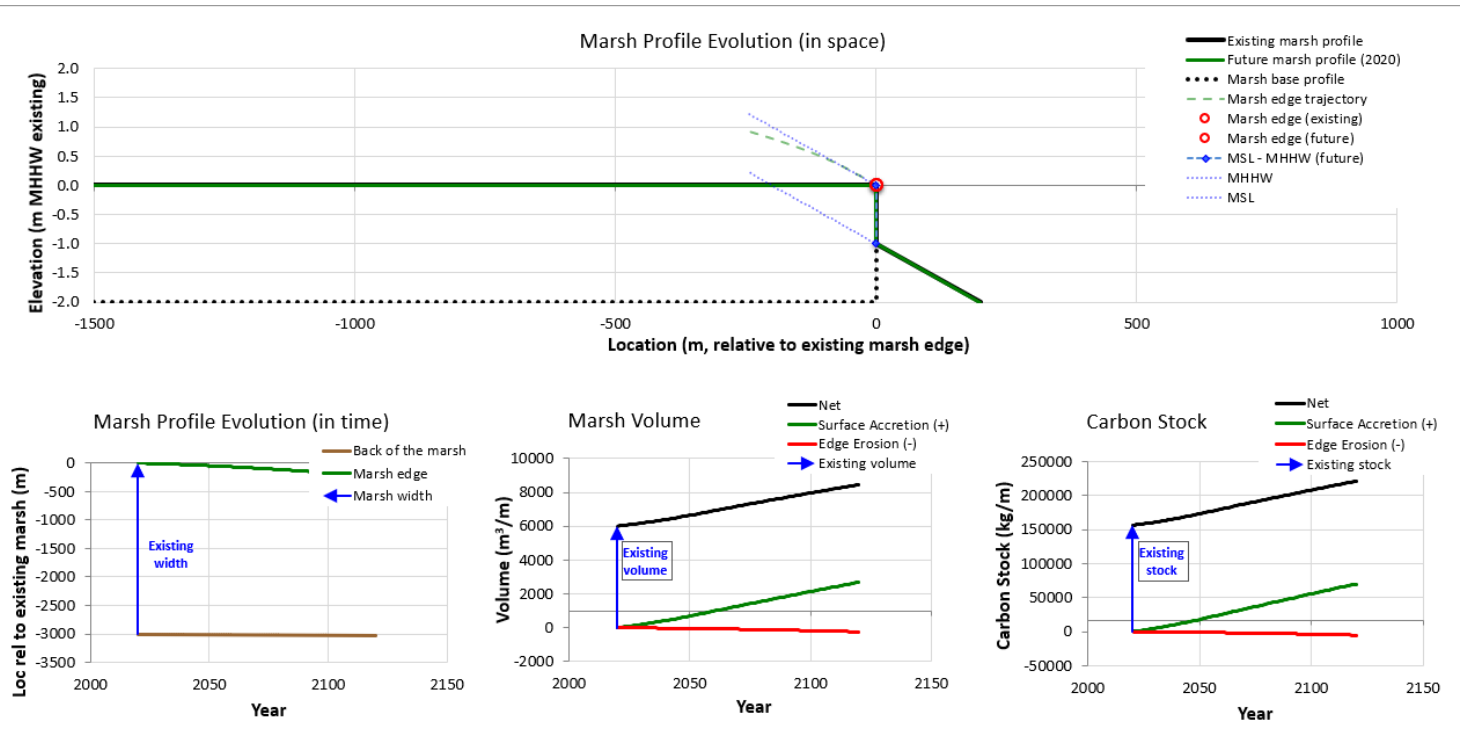
Figure 1: Illustration of the model setup. Within the model, initial mangrove surface elevation (and hence elevation capital) is set by adjusting tidal range. Here the mangrove surface is 1 mMSL (m above mean sea level) and an accretion rate of 10 mm yr -1 maintains vegetation at or just above the mangrove drowning elevation by year 2020. Retreat of a 0.5 m high cliff mangrove edge by 609 m with sea level rise over a century leads to release of soil carbon, 80% of which is assumed to be mineralized.
