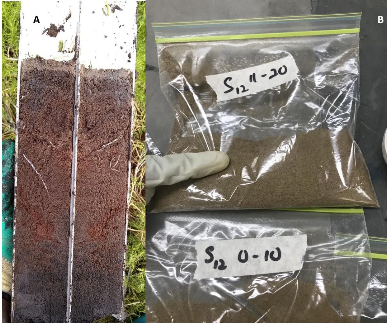
Figure 3 Example of sediment (Short Core) extracted from the site (A) and how it is bagged into 0 – 10 cm, 11 – 20 cm etc. (C).
