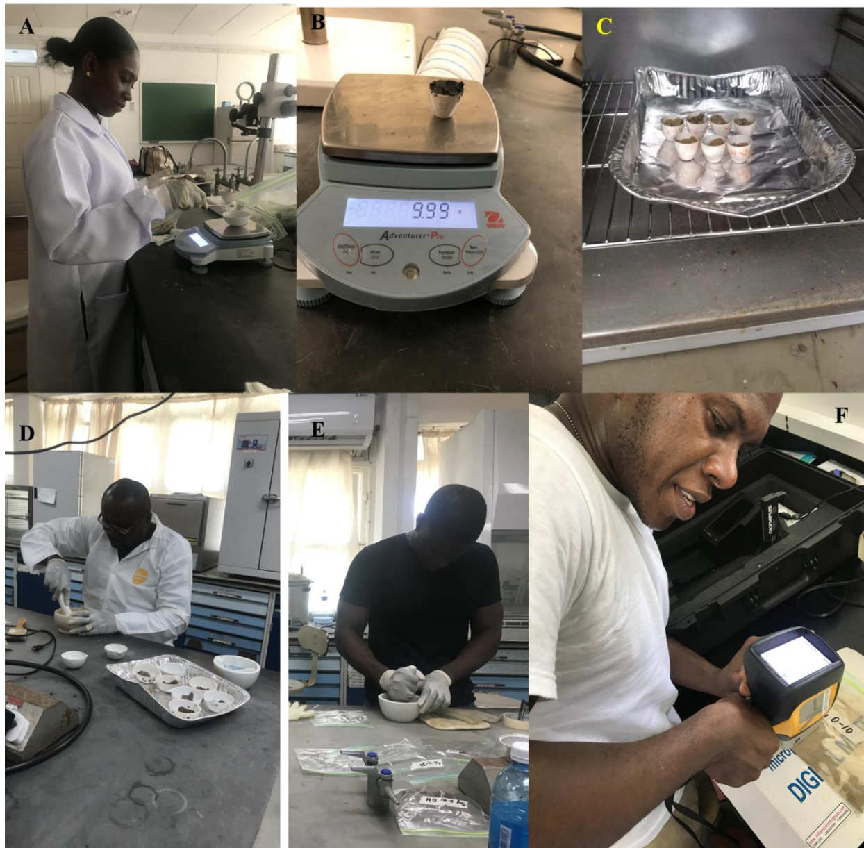
Figure 8 Example of sediment preparation in the lab after the fieldwork. Weighing the sediments (A and B) before being put into the oven for oven dried for three days (C). The dried samples were pulverised into fine powder using an agate mortar and pestle (D and E). Each pulverised ground sample were then weighed and measured prior to analysis using Handheld X-ray Fluorescence Spectrometry (XRF) to determine the major oxide and trace element composition of sediment samples (F).
