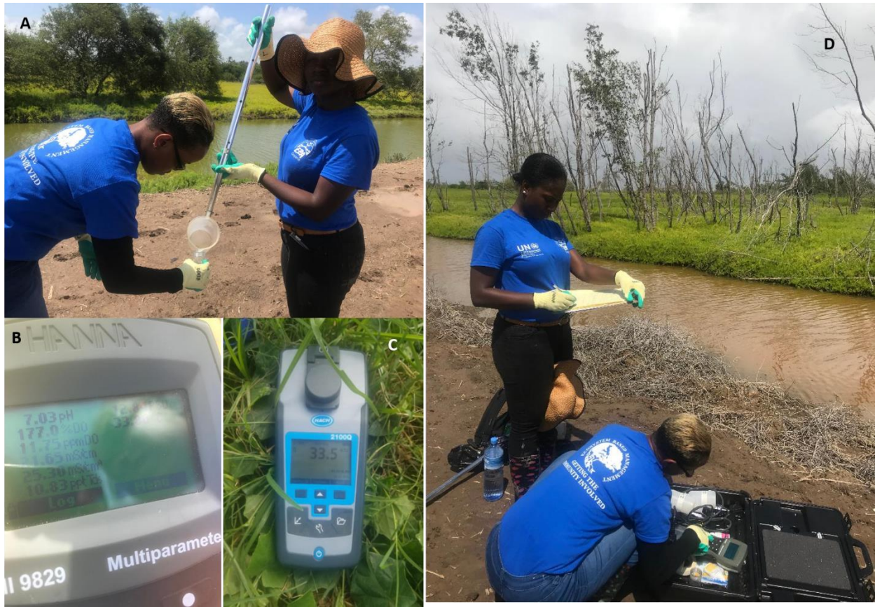
Figure 5 Example of surface water sampling on the field for multiparameter testing and labs (A) Hanna HI9829 multi-parametre probe used at the field (B) and HACH 2100P turbidimeter (C). Examining water quality parameter using HI9829 multi-parameter probe on the field and recording the observations (D).
